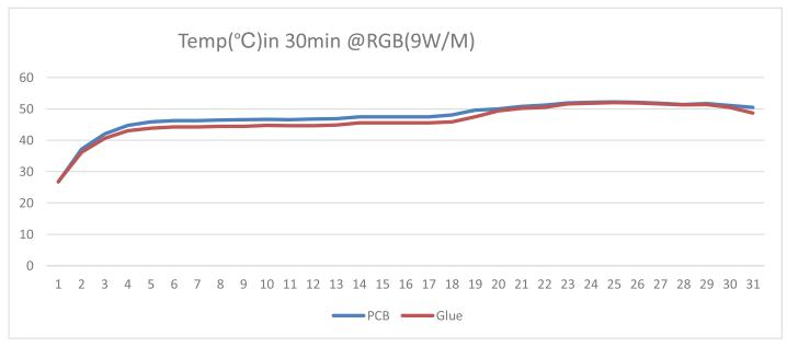
The above curves indicate the temp. changing in glue & PCB within 30 minutes after powering on, under the ambient temperature of 25°C. The following charts shows the parameters on each meter based on 8M length.
