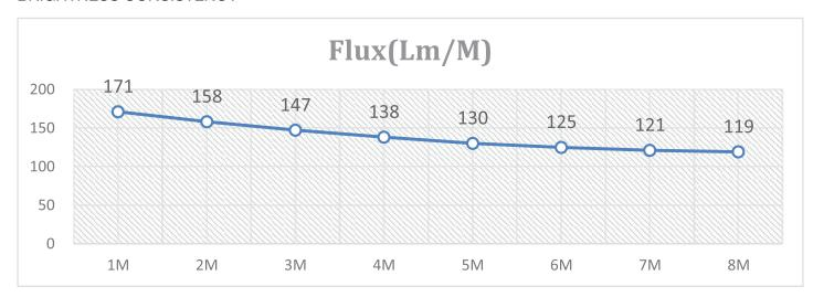
From above chart, please connect 8M at most by one-end power to keep brightness consistency
